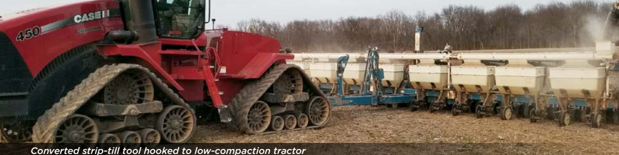
Converted strip-till tool hooked to low-compaction tractor
